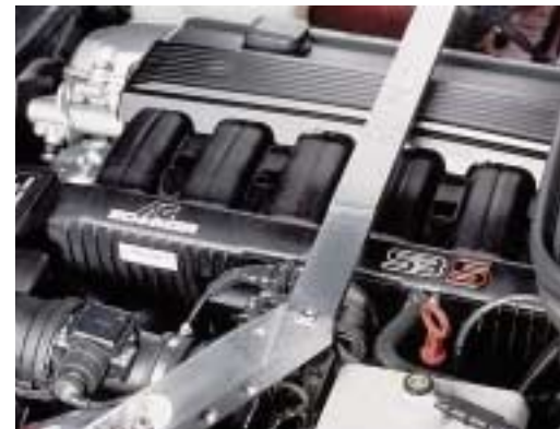
AC Schnitzer intake manifold kit Z3 S for BMW Z3 2.8 with M52 engine, power increase 18kW (25HP), strut brace for Z3 in preparation
