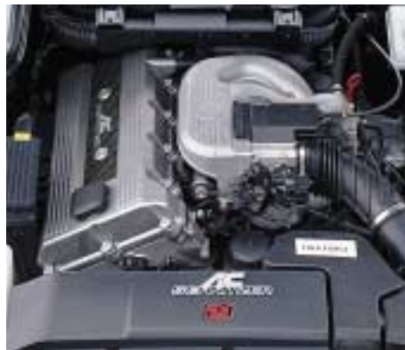
AC Schnitzer Z3 2.1 power plant for BMW Z3 1.8 with M43 engine, power 108 kw (147 HP). AC Schnitzer Z3 2.1 power plant for BMW Z3 1.9 with M44 engine, power 129 kw (175 HP)
