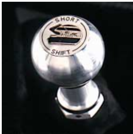
AC Schnitzer "Short Shift" sports gear change - shorter selector travel as fitted to Touring Cars
