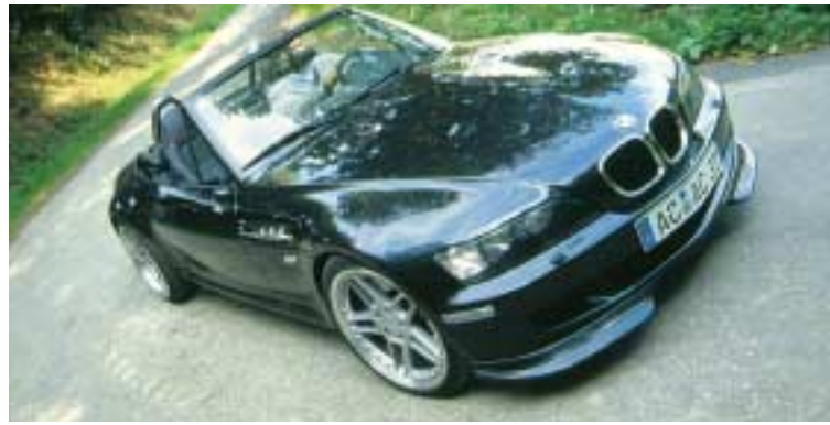
The AC Schnitzer front skirt with integral fog lights and enlarged air inlets to guarantee optimum aerodynamic performance
