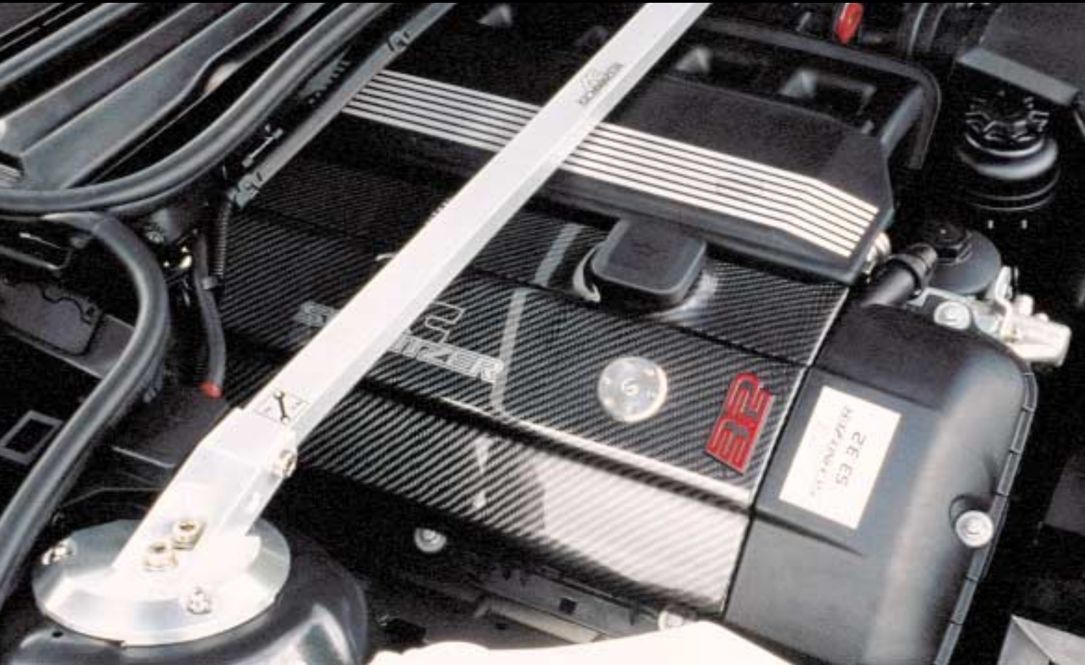
AC Schnitzer Z3 3.2 engine for BMW Z3 2.8 with M52 TU engine, power increase 31kW (42 HP). Strut brace for Z3 in preparation
