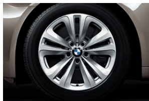
□ 18" light alloy wheels Double-spoke 234 , 8 J x 18, 245/50 R 18 Y tyres (standard on 740i/Li, 750i/Li and 740d). Also available as a complete winter wheel-and-tyre set in the Original BMW Accessories range*.
