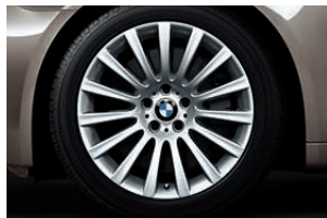
□ 19" light alloy wheels Multi-spoke 235 with mixed tyres, 8.5 J x 19 wheels and 245/45 R 19 Y tyres at the front, 9.5 J x 19 wheels and 275/40 R 19 Y tyres at the rear (standard on 760i/Li). Also available as a complete winter wheel-and-tyre set in the Original BMW Accessories range*.
