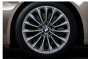
□ 19" light alloy wheels Radial-spoke 252 , forged, with mixed tyres, 8.5 J x 19 wheels and 245/45 R 19 Y tyres at the front, 9.5 J x 19 wheels and 275/40 R 19 Y tyres at the rear.
