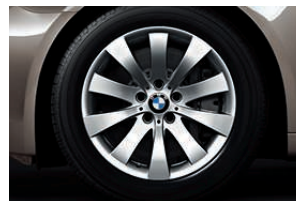
□ 18" light alloy wheels Star-spoke 250 , 8 J x 18, 245/50 R 18 Y tyres. Also available as a complete winter wheel-and-tyre set in the Original BMW Accessories range*.
