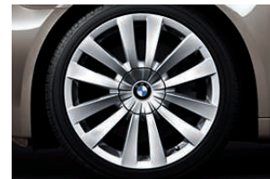
□ 20" light alloy wheels Double-spoke 253 with mixed tyres, 8.5 J x 20 wheels and 245/40 R 20 Y tyres at the front, 10 J x 20 wheels and 275/35 R 20 Y tyres at the rear.
