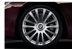
20" light alloy wheels V-spoke 374 I, forged. Front 8.5 J x 20, 245/35 R 20; rear 9 J x 20, 275/30 R 20.
