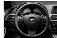
M leather steering wheel , multifunction, with shift paddles for eight-speed Sport transmission.
