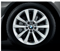
□ 18" BMW light-alloy wheels V-spoke 328 with runflat tyres, 8 J x 18, 245/45 R 18 tyres (standard on 550).
