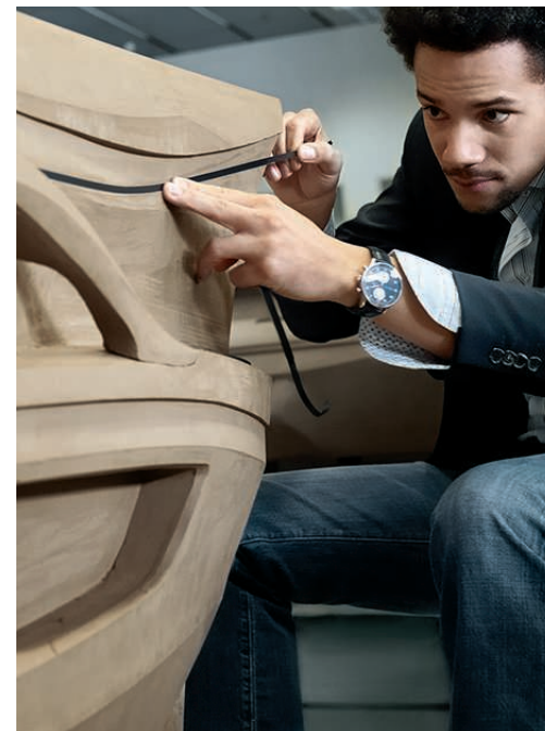
Interior designer Oliver Heimer checking the lines and dimensions of the body on the clay model.
