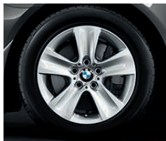
□ 17" light-alloy wheels star-spoke 327 with runflat tyres, 8 J x 17, 225/55 R 17 tyres.
