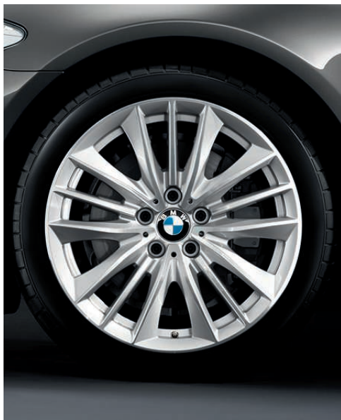
□ 19" light-alloy wheels W-spoke 332 with mixed runflat tyres, 8.5 J x 19, 245/40 R 19 tyres at the front, 9 J x 19, 275/35 R 19 tyres at the rear.
