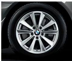
■ 17" light-alloy wheels V-spoke 236 , 8 J x 17, 225/55 R 17 tyres (standard on 520i, 528i, 530i, 535i, ActiveHybrid 5, 520d, 525d, 530d and 535d).
