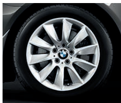
□ 18" light-alloy wheels turbine styling 329 with mixed runflat tyres, 8 J x 18, 245/45 R 18 tyres at the front, 9 J x 18, 275/40 R 18 tyres at the rear.
