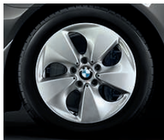
□ 17" light-alloy wheels Streamline 363 with runflat tyres, 8 J x 17, 225/55 R 17 tyres (standard on 520d EfficientDynamics Edition, without runflat tyres).
