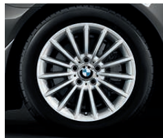
□ 18" light-alloy wheels radial-spoke 237 with runflat tyres, 8 J x 18, 245/45 R 18 tyres.
