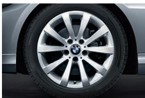
□ 17" light-alloy wheels V-spoke styling 285 with runflat tyres, 8 J x 17, 225/45 R 17 tyres (standard on 325i xDrive, 330i, 335i, 325d, 330d and 335d).
