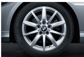
□ 17" light-alloy wheels star-spoke styling 286 with mixed runflat tyres, 8 J x 17, 225/45 R 17 tyres at the front, 8.5 J x 17, 255/40 R 17 tyres at the rear.
