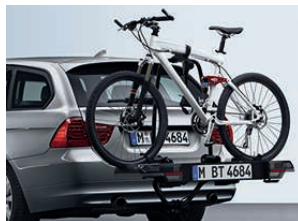
Rear carrier for trailer tow hitch , for up to three bicycles.
