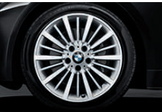
□ 18" light-alloy wheels multi-spoke 416, highly polished, with runflat tyres, 8 J x 18, 225/45 R 18 tyres (standard on 328i and 335i).
