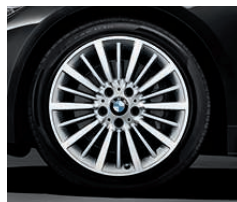
□ 18" light-alloy wheels multi-spoke 416 , highly polished, 8 J x 18, 225/45 R 18 tyres (available only in conjunction with the Luxury Line, standard on 328i and 335i).
