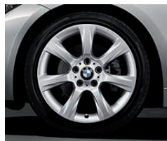
18" light-alloy wheels star spoke 396 , 8 J x 18, 225/45 R 18 tyres.
