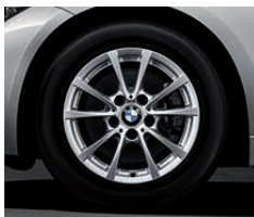
16" light-alloy wheels V-spoke 390 , 7 J x 16, 205/60 R 16 tyres (standard on 320i and 320d).
