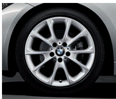
18" light-alloy wheels V-spoke 398 with mixed tyres, 8 J x 18, 225/45 R 18 tyres at the front, 8.5 J x 18, 255/40 R 18 tyres at the rear.
