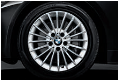
■ 17" light-alloy wheels multi-spoke 414 with runflat tyres, 7.5 J x 17, 225/50 R 17 tyres.
