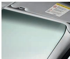
□ Windscreen with grey shade band prevents drivers from being dazzled by the sun.
