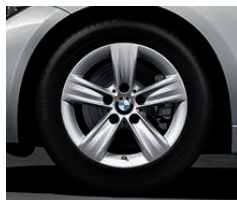
16" light-alloy wheels star spoke 391 , 7.5 J x 16, 225/55 R 16 tyres.
