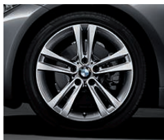
□ 18" light-alloy wheels double-spoke 397 , in bi-colour Ferric Grey, highly polished, 8 J x 18, 225/45 R 18 tyres (available only in conjunction with the Sport Line, standard on 328i and 335i).
