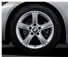
17" light-alloy wheels star spoke 393 , 7.5 J x 17, 225/50 R 17 tyres.
