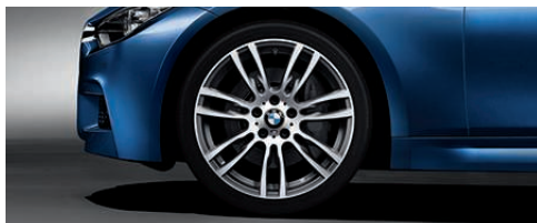
□ 19" M light-alloy wheels double-spoke 403 M in bi-colour Ferric Grey, highly polished, with mixed tyres, 8 J x 19, 225/40 R 19 tyres at the front, 8.5 J x 19, 255/35 R 19 tyres at the rear (only available in conjunction with M Sport package). □ M Sport brake, 2 fixed-caliper brake, front/rear in dark blue, larger brake disc and coloured M logo (only available in conjunction with M Sport package).
