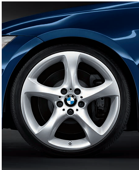
□ 19" light-alloy wheels star-spoke 230 i with mixed tyres, 8 J x 19, 225/35 R 19 tyres at the front, 9 J x 19, 255/30 R 19 tyres at the rear.
