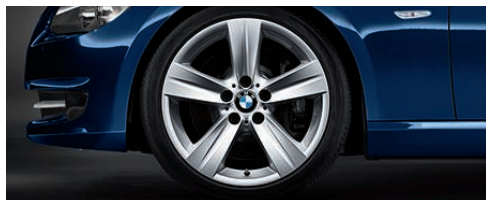
□ 18" light-alloy wheels star-spoke 189 with mixed tyres, 8 J x 18, 225/40 R 18 tyres at the front, 8.5 J x 18, 255/35 R 18 tyres at the rear.
