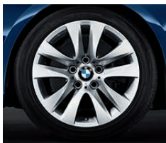
□ 17" light-alloy wheels V-spoke 338 , 8 J x 17, 225/45 R 17 tyres (standard on 330i and 330d).
