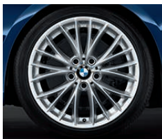
□ 18" light-alloy wheels V-spoke 342 with mixed tyres, 8 J x 18, 225/40 R 18 tyres at the front, 8.5 J x 18, 255/35 R 18 tyres at the rear.
