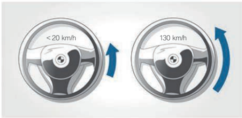
□ Servotronic adjusts the steering power to suit the current speed. It ensures steering transmission that is direct, precise and won't tire you out. In addition, Servotronic makes your drive more comfortable by reducing the effort required to turn the wheel and providing maximum manoeuvrability while parking.
