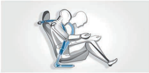
■ BMW restraint system for driver and front passenger. A combination of three-point seatbelts, pyrotechnic belt tensioners and belt force limiters provides the best possible restraint in the event of a collision.
