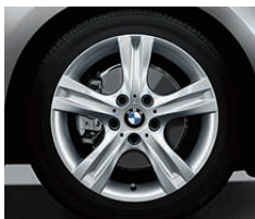
□ 17" light alloy wheels Star-spoke 262 with mixed runflat tyres, front 7 J x 17 with 205/50 R 17 tyres, rear 7.5 J x 17 with 225/45 R 17 tyres (not for 135i).
