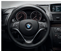
□ Sport leather steering wheel with multifunction buttons (diameter 369 mm), chrome inlay 2 , three spokes, including multifunction buttons for the remote control of radio or optional telephone (standard with the 125i, 135i and 123d).
