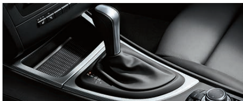
□ Six-speed automatic transmission Steptronic (shown here with non-smoker package) with Adaptive Transmission Management. Allows for very fast, precise gearshifts for maximum dynamic performance (not for 135i).
