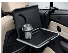
Travel & Comfort system , folding table, mounts on the front seat headrest pillars.
