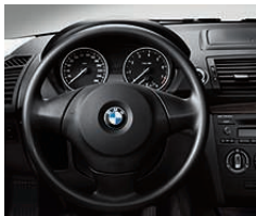
■ Standard steering wheel (diameter 375 mm), three-spoke.
