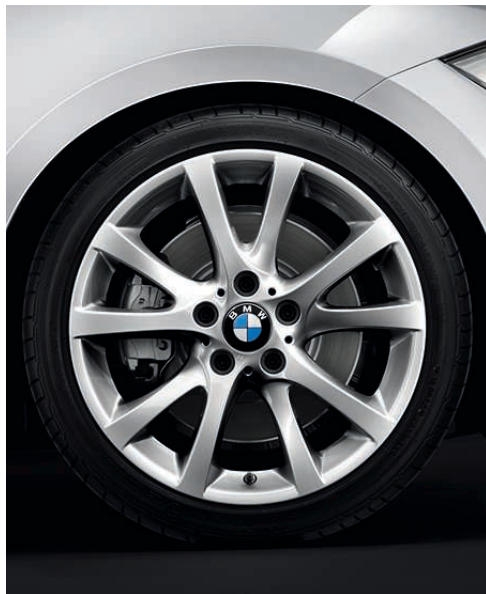
□ 18" light-alloy wheels V-spoke 372 with mixed runflat tyres, 7.5 J x 18 with 215/40 R 18 tyres at the front, 8.5 J x 18 with 245/35 R 18 tyres at the rear.
