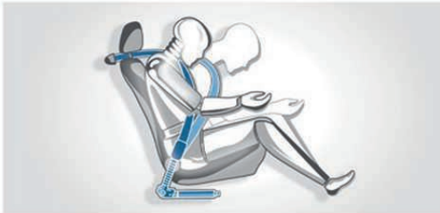
BMW restraint system for the driver and front passenger, comprises three-point seat belts featuring belt tensioners and belt force limiters. So in the event of a collision, passengers are held safely in their seats. The seat belt buckles in the rear are coded to avoid them being incorrectly fastened.
