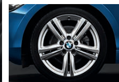
18" M light alloy wheels Star-spoke 386 M with mixed tyres, front 7.5 J x 18 with 225/40 R 18 tyres, rear 8 J x 18 with 245/35 R 18 tyres.
