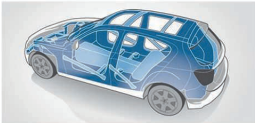
Passenger cell . The system of members and nodes in the functional body structure combined with the strategic deployment of high-strength materials delivers maximum passive safety in front, side or rear crashes. Defined deformation zones mean that the body structure can absorb impact energy, increasing passenger protection.
