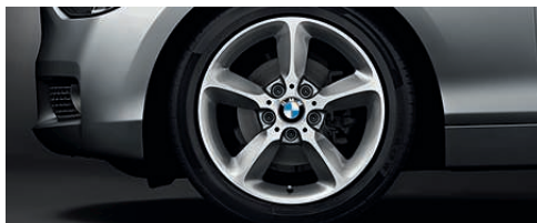
□ 17" light alloy wheels Star-spoke 382 , in bi-colour Space Grey metallic and gloss-lathed, with mixed tyres, front 7.5 J x 17 with 225/45 R 17 tyres, rear 8 J x 17 with 245/40 R 17 tyres.
