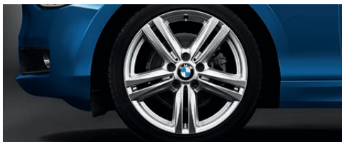
□ 18" M light alloy wheels Star-spoke 386 M with mixed tyres, front 7.5 J x 18 with 225/40 R 18 tyres, rear 8 J x 18 with 245/35 R 18 tyres (only available in conjunction with the M Sport package).
